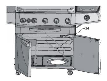
a) Insert the tank clip (24) into the holes on the gas tank seat.
