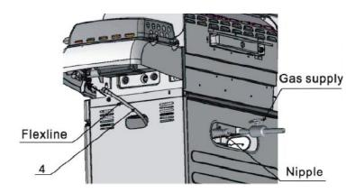
a) Connect the natural gas hose (4) with the side burner valve by screwing the nut on end of the hose.
